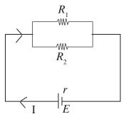
$$R_{f} = \frac{R_{1}R_{2}}{(R_{1} + R_{2})}$$
