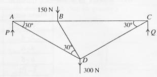
Draw a stress diagram using Bow's notation and hence, find the stresses in all the rods and state whether they are tensions or thrusts.
