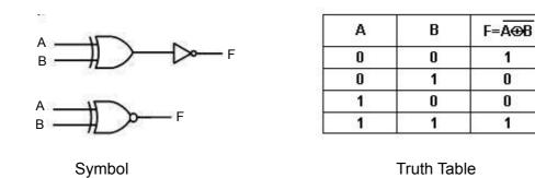
The output of this gate is the negation of the output of XOR logic gate.
