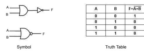
The output of this gate is the negation of the output of the OR logic gate.
