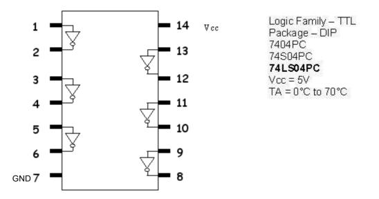
By constructing the above circuit on an Electronic Project Board, using an Integrated circuit (IC), light emitting diode and a power supply, the action of a NOT gate could be studied.
