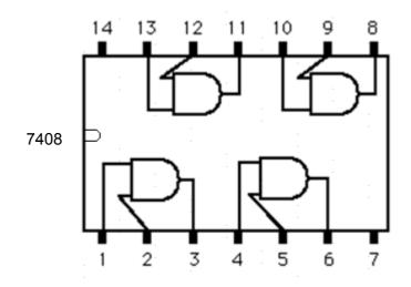
By building the above circuit on an Electronic Project Board using an Integrated Circuit, light emitting diode and power source, the action of an AND gate can be studied.
