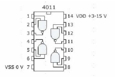
By building the above circuit on an Electronic Project Board using an Integrated Circuit, light emitting diode and power source, the action of an NAND gate could be studied.
